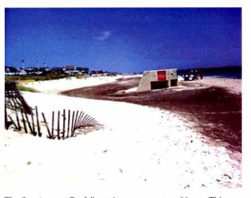
The Sea Avenue Outfall continues to cause problems. This past summer there were at least three discharges on to the sand after rain storms. The discharge in mid July left a deposit on the sand which ran approximately IOOO ft. northward along the two adjacent beaches and about IOO feet south along the municipal beach.
